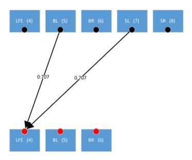
The above example mixes the side and rear left surround channels of a 7.1 file to LFE of a 5.1 file (the figure only shows the last few channels in the diagram). The ffmpeg pan filter will show the channel mix as: c3=0.707\*c4+0.707\*c5
